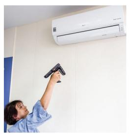
Automated inventory of assets with the use of a long-range mobile RFID chip scanner.
